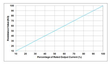
5. 1 ~ 10V dimming function for output current adjustment (Typical).
