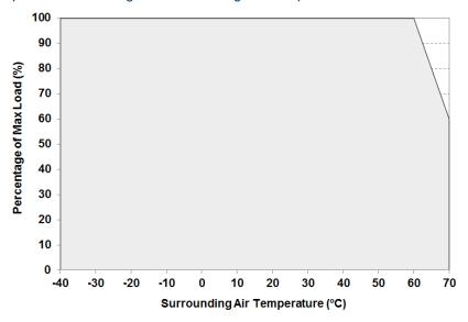
Fig. 1 De-rating for All Mounting Orientation (All Models) > 60°C de-rate power by 4% / °C
