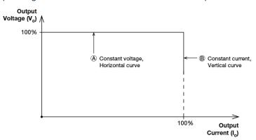
A typical LED power supply is able to either work in "constant voltage mode (CV) or constant current mode (CC)" to drive the LEDs. Delta's LNE drivers integrate CV+CC characteristics; so operation in CV mode (with external LED driver), in region (A) or CC mode (direct drive, at area (B)).
